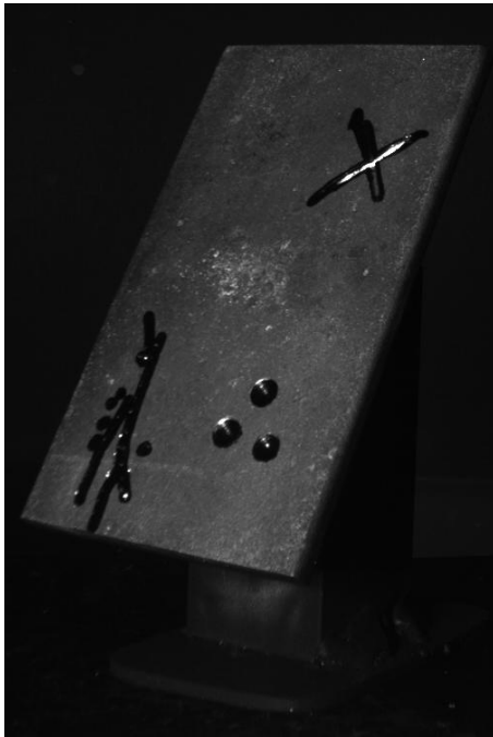
Scanner photograph of object before scan. Bottom left corner shows surface abrasion, bottom right shows divots and the top right simulates a crack
