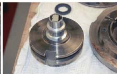
A Proof 2012-S Benjamin Harrison Presidential obverse die is shown, left, in the die housing surrounded by the three-piece segmented collar containing the edge inscriptions. At right, the same die is shown removed from the die housing.
