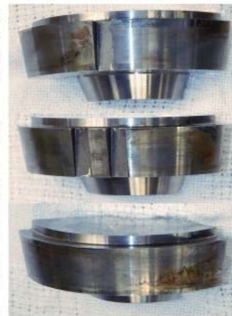
The three pieces of the segmented collar are coded by number of slots: having no slot, bottom; two slots, center; and one slot, top. The coding ensures that only one of each of the three collar segments is used and that they are properly seated in correct order in the die housing.
