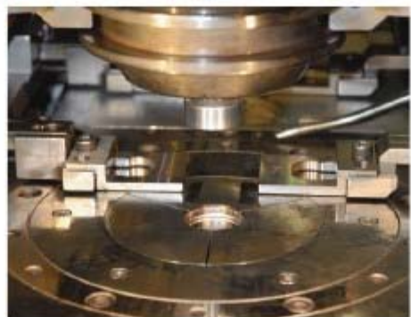
On the press, the upper, or hammer die, for the Proof Presidential dollars is the reverse, and the bottom, or anvil die, is the obverse.
