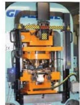
All Coin World images by Paul Gilkes. A Newton Press Die Inspection System mounted on the front of a Gräbener coinage press at the San Francisco Mint is being used to inspect for installation of the correct dies in the proper die alignment.
