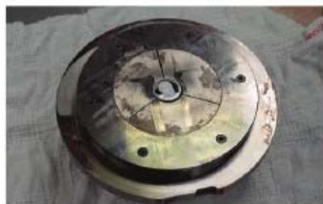
A Proof 2012-S Benjamin Harrison Presidential obverse die is shown, left, in the die housing surrounded by the three-piece segmented collar containing the edge inscriptions. At right, the same die is shown removed from the die housing.
