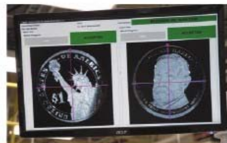
The inspection screen digitally scans the dies to ensure the proper dies are placed correctly in the hammer or anvil die position and are in proper die alignment before production begins.
